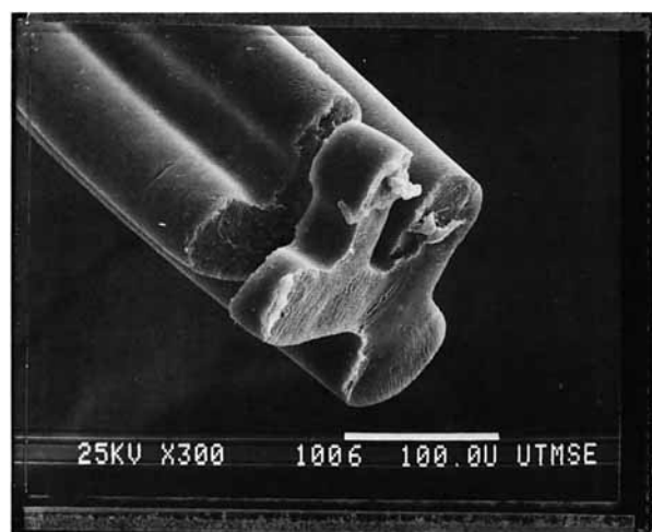
Figure 14 SEM photograph of a polystyrene fiber formed by spraying a 12.8% polystyrene in toluene solution through a 151 μm nozzle into liquid methanol at 22°C and with a Δ P = 65.5 bar.
